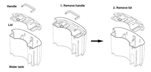
Please note, located inside the water tank is a float. It is essential this float is NOT removed from the water tank. The float measures the level of water in the water tank and triggers the sensor to turn the dehumidifier off when the water tank is full.
