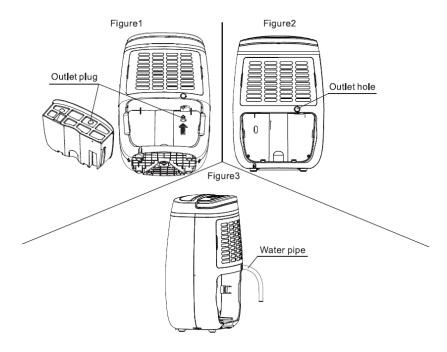
In order to use continuous drainage, remove the water tank from the unit. Remove the rubber bung from the water tank and insert it into the spout which drips into the water tank. Snip the circular disc on the back of the unit (to the bottom right of the filter) and push the 12mm hose through the hole securing it to the internal outlet pipe. Once the hose is in place, put the water tank back into the unit (for continuous drainage to work, the water tank must always be in place).
