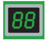
Once the target humidity level has been reached (is more than 3% below) the dehumidifier will go to sleep for half an hour and the reading on the display may increase significantly, this is because the dehumidifier is reading its internal humidity level, it is not showing the external relative humidity level in the environment (see page 14 for more information).
