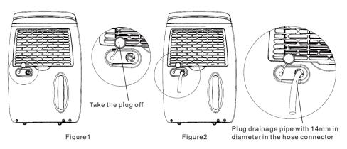
In order to use continuous drainage, take the plug off the back of the unit and push the 14mm hose through the hole securing it to the internal outlet pipe (for continuous drainage to work, the water tank must always be in place).
